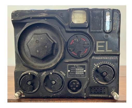
Author John Harris's 1943 model of the Lorenz FuG10 EL [long wave] radio transceiver, designed as a blind landing aid for the German air force.
